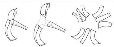
A network structure consists of ribs. All ribs have a triangular cross section, that is made out of three bespoke curved sheets of steel.
